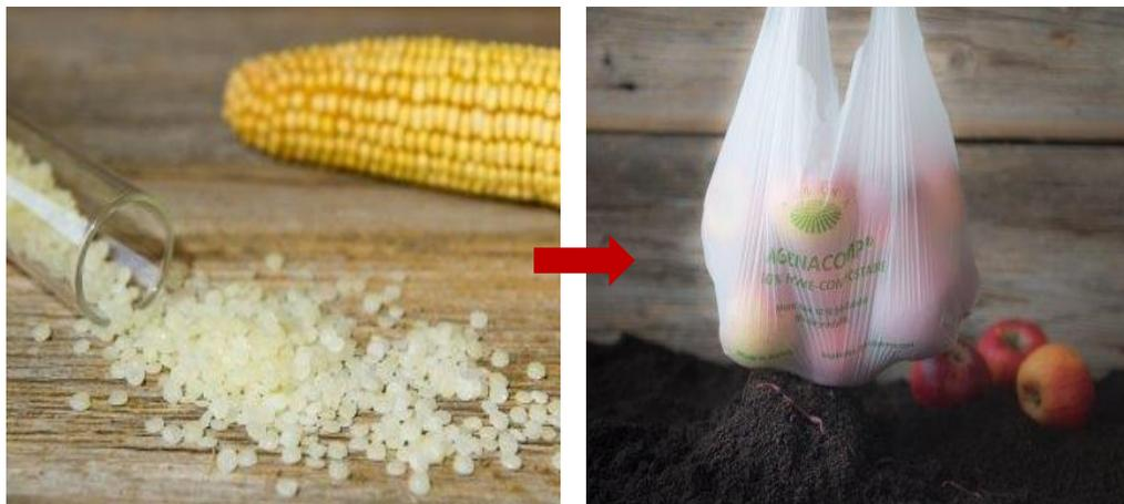
Thermoplastic starch as a basis for compounds for plastic bags, foils, injection molding elements
